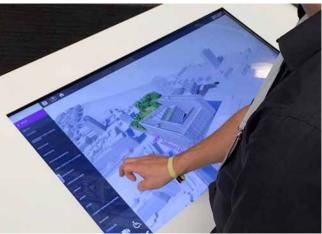
Projected capacitive technology enables touch points to be sensed through a protective layer in front of the display, this means the table top can have an almost completely flat surface.
