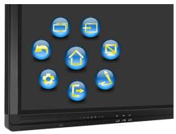
Onscreen menu allows you to change volume, change video input, freeze the screen, annotate, and turn off the screen. These options are also accessible from the buttons on the side of the screen.
