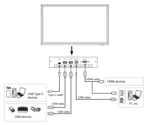
Connect TOUCH OUT with USB cable to PC USB port.
