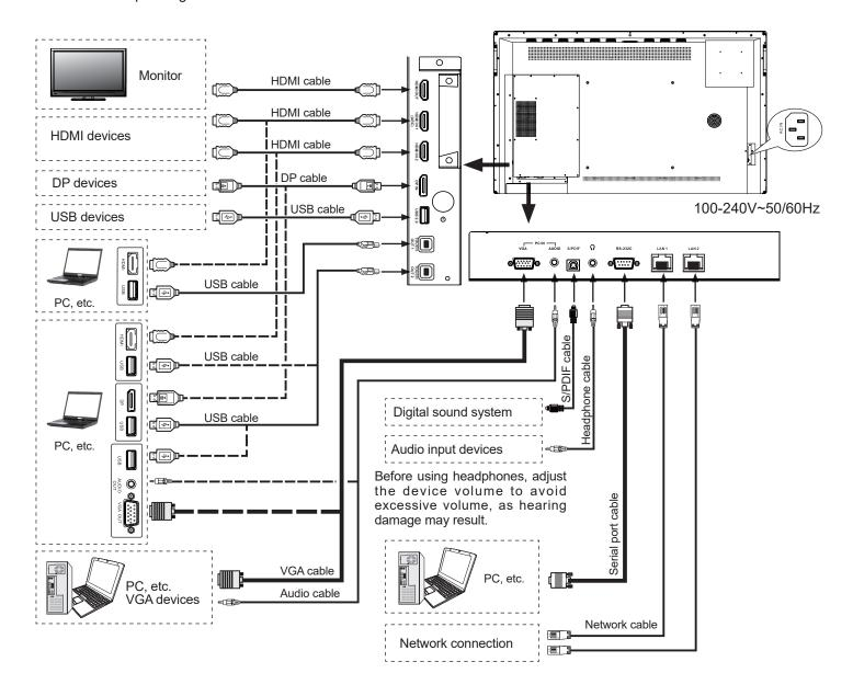
Connect TOUCH OUT with USB cable to PC USB port.
